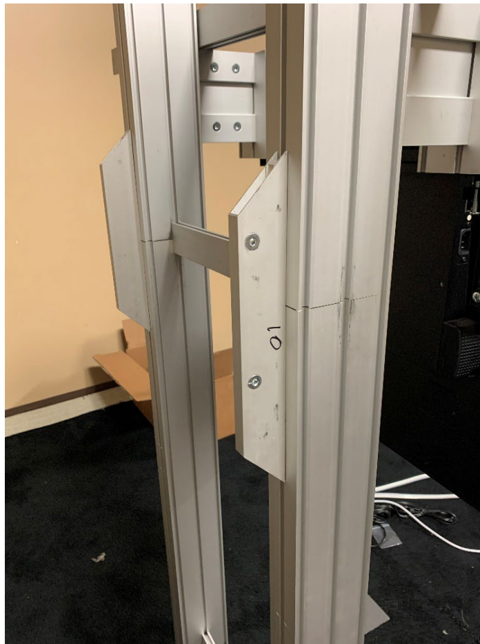
(2) AF16 (B4): add to back supports of mount and tighten seam
