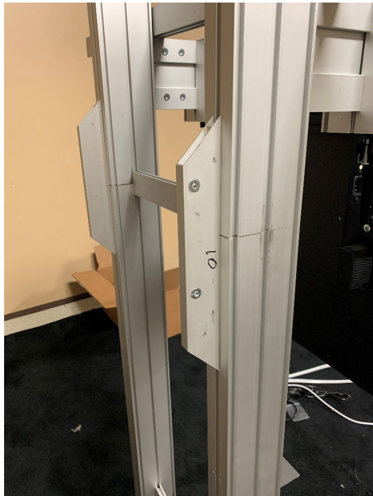
(2) additional feet (B3) added to inside of monitor mount for stability
