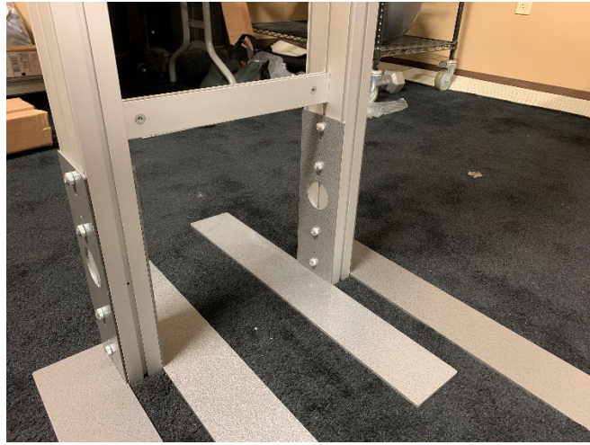
(2) additional feet (B3) added to inside of monitor mount for stability
