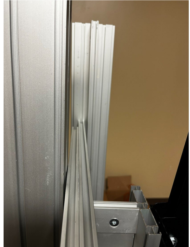
Cams attach on inside channel closest to tv mount bean on 4" extrusion.
